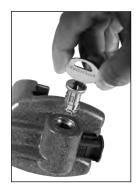
With the locking member pushed down, the sliding bolt can be removed from the lock completely. While holding the locking member down, use a finger to hold it in place from the top while reinserting the plug. The plug should have the removal tool in it and the rod extending from the back toward the bottom of the lock when inserted
